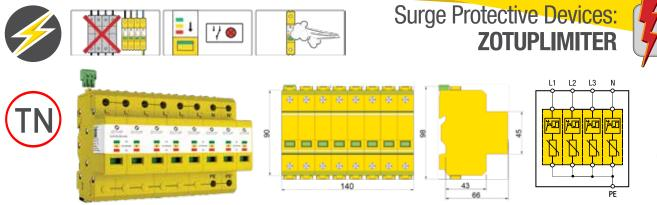
L 25/100 230 t ff 4 is a ready to install assembly of four voltage limiting SPDs providing four modes of protection, typically installed at the origin of the installation, e.g. in the Main Distribution Board (MDB), for three-phase plus neutral 230/400 V TN-systems, with the following features and benefits:
