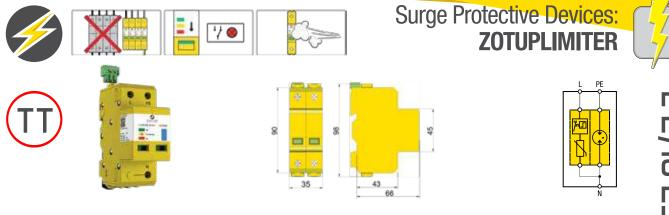
L 2/10 230 ff 1+1 is a ready to install assembly of a voltage limiting and a voltage switching SPD providing two modes of protection, typically installed in Sub Distribution Boards (SDBs) for single-phase 230 V TT-systems where connection type CT2 (1+1) is required according to HD 60364-5-534, with the following features and benefits:
