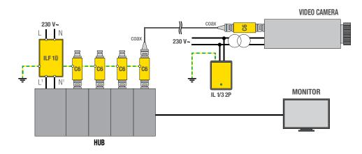
C 6 is an SPD for the protection of CCTV circuits, typilcally installed on each line near to the HUB and close to the video cameras, providing the following features and benefits:
