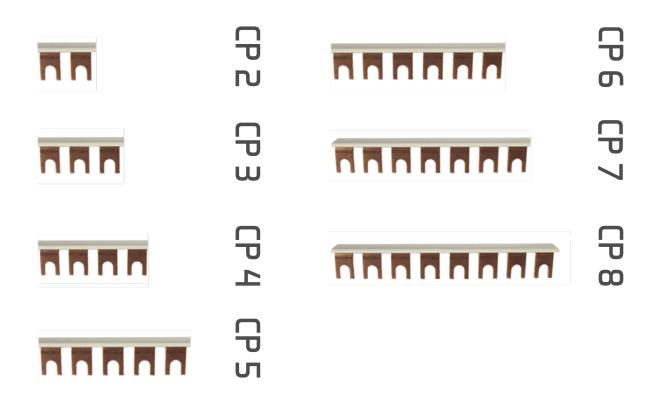
**CP2 to CP8 are fork-type busbars with 2 up to 8 connection points. Typical application: to provide a common PE connection for several SPDs.** In TT system applications these busbars can also be used to provide a common neutral point connection to N-PE SPDs type I 12, I 52 and I 100.
