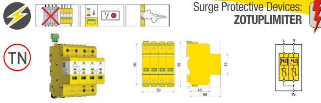
L 25/100 230 t ff 2 is a ready to install assembly of two voltage limiting SPDs providing two modes of protection, typically installed at the origin of the installation, e.g. in the Main Distribution Board (MDB), for single-phase 230 V TN-systems, with the following features and benefits:
