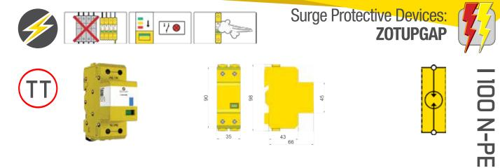
I 100 N-PE is a voltage switching SPD providing a single mode of protection, typically installed in TT-systems between neutral conductor N and protective earth PE, where connection type CT2 (1+1 or 3+1) is required according to HD 60364-5-534, e.g. in the Main Distribution Board (MDB), with the following features and benefits:
