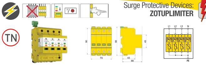
L 7/30 230 ff 4 is a ready to install assembly of four voltage limiting SPDs providing four modes of protection, typically installed at the origin of the installation, e.g. in the Main Distribution Board (MDB), for three-phase plus neutral 230/400 V TN-systems, with the following features and benefits:
