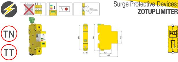
L 2/10 230 ff is a voltage limiting SPD providing a single mode of protection, typically installed in Sub Distribution Boards (SDBs), in TN-systems or in TT-systems in combination with N-PE SPD model I 52 or I 12 and where connection type CT2 (3+1 or 1+1) is required according to HD 60364-5-534. It provides the following features and benefits:
