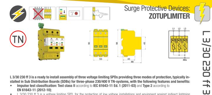
L 3/30 230 ff 3 is a ready to install assembly of three voltage limiting SPDs providing three modes of protection, typically installed in Sub Distribution Boards (SDBs) for three-phase 230/400 V TN-systems, with the following features and benefits: Impulse test classification: Test class II according to IEC 61643-11 Ed. 1 (2011-03) and Type 2 according to •
